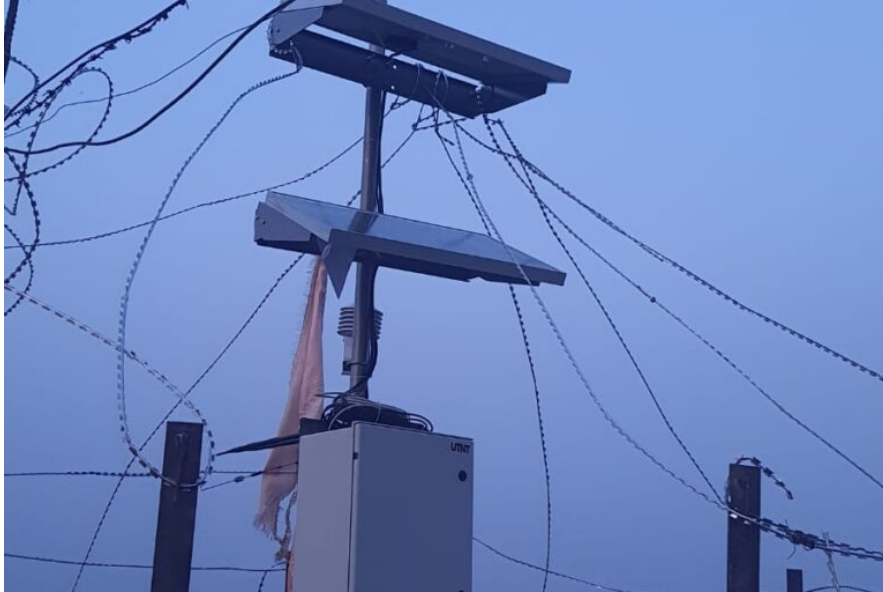
A PhenoMet station. Such stations record and understand phenological processes and their relation to weather conditions. Photo by Ami Kumar.
